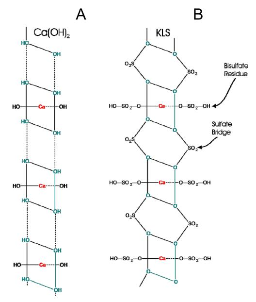
"A" - Edge of a calcium hydroxide crystal with two thirds of the calcium ions removed.
